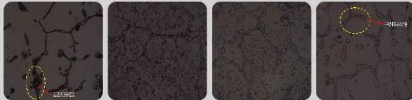
Microstructural Examination of HP 50 by Replica
