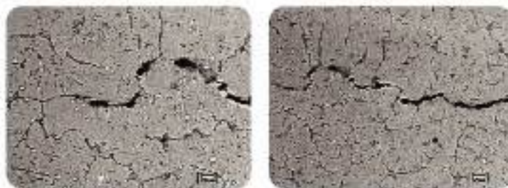
Intergranular cracking of Inconel 800 at high temperature(failure by creep)
