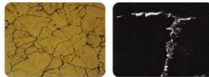
Sensitized microstructure of austenite stainless steel (Optical Microscopy and SEM)
